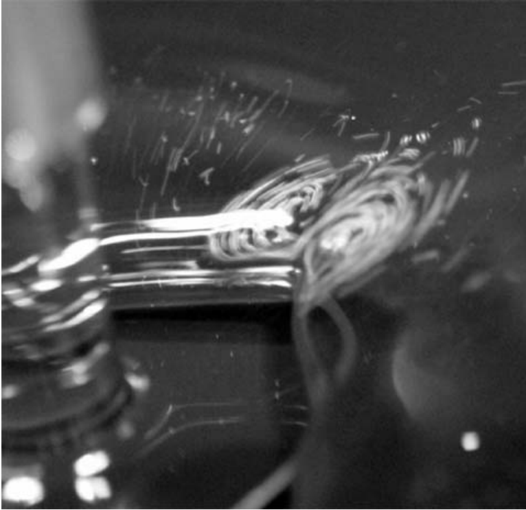
FIGURE 5. A streak image illustrating bubble tracks in the neighbourhood of the corners of the hydraulic jump. The shutter speed was 1/100 s; the image thus illustrates clearly the high speed of the flows. Note the regions of recirculation adjoining the jump and the vigorous vortices adjoining the corners.
